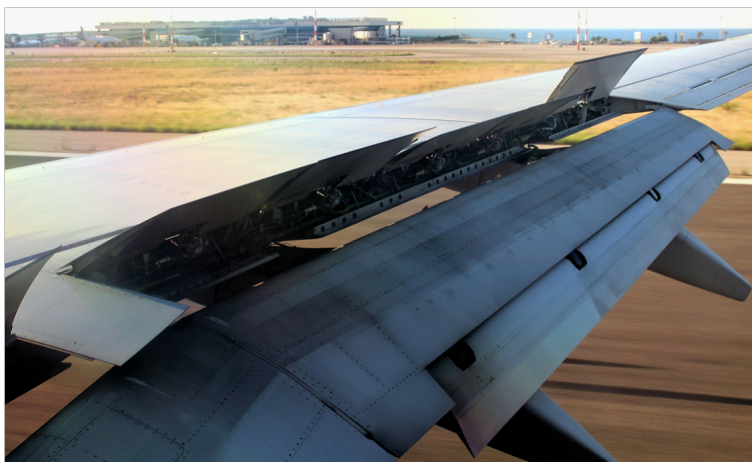
Figure 4: Aircraft flap section made of panels bonded too honeycomb structure
