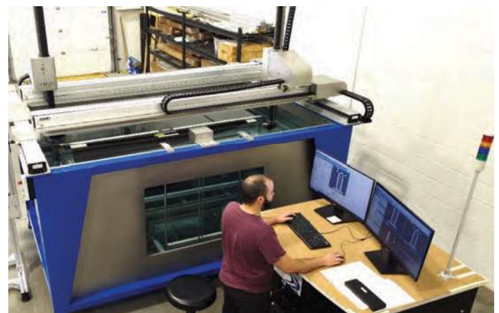
Figure 2: Scan3D 10-axis Ultrasonic Immersion System
